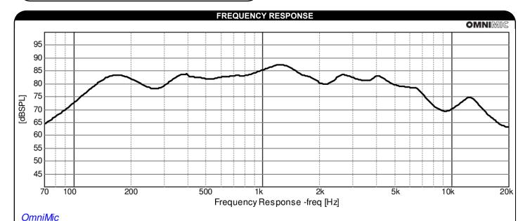
1/3<sup>rd</sup> octave smoothing - measurement taken with transducer adhered off-center on a 12" x 12" x 1/2" foam core board in an infinite baffle setup.
