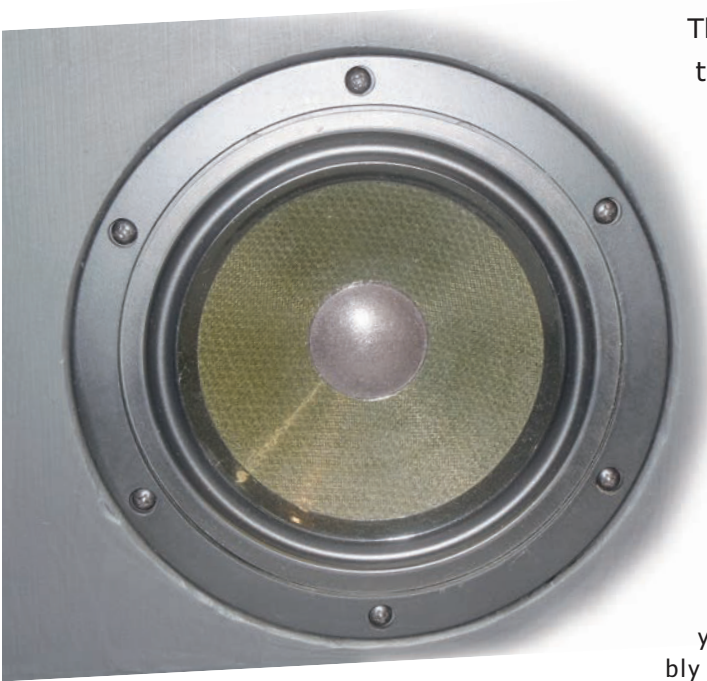
Photo 1: The Eton 7" drive has a light rigid cone made of a Nomex honeycomb sandwiched between two Kevlar layers for true pistonic behavior.
