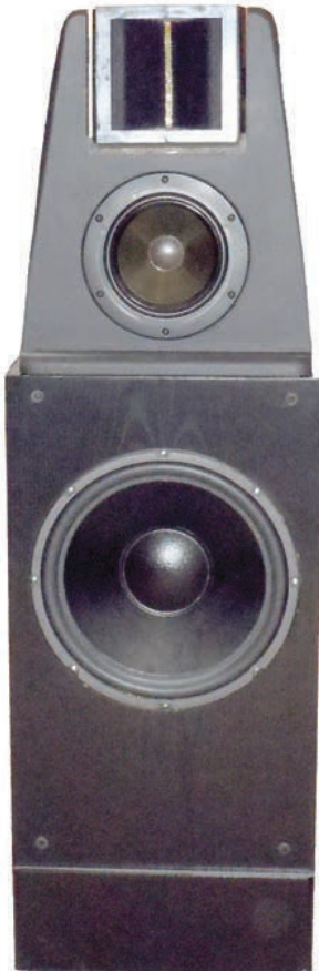
Photo 4: The original speaker used an HSU 12" bass driver, which is shown without the grille.
