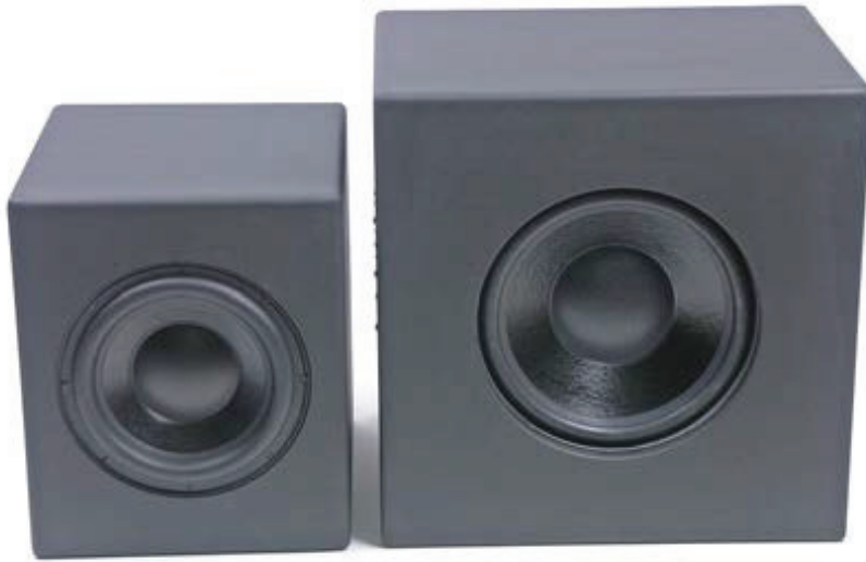
Photo 5: The differing sizes of the finished 2-ft 3 and 5-ft 3 enclosures with the drivers mounted are shown for comparison.
