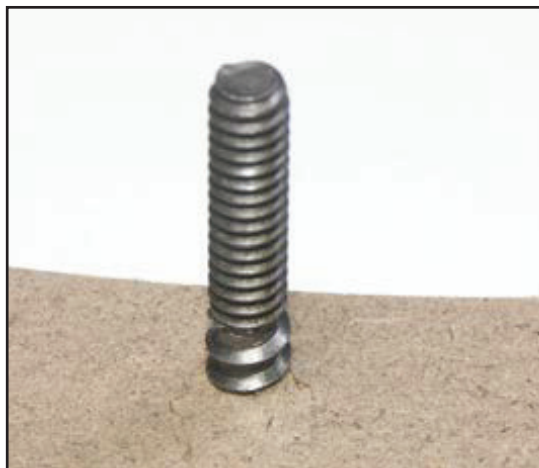
Photo 3: The hanger bolt is installed in MDF near the driver opening.
