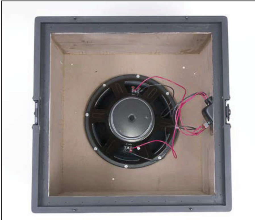
Photo 4: The DVC 15" driver has been mounted and wired.
