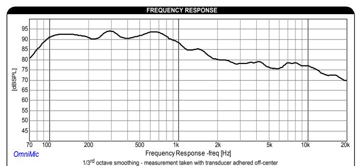
on a 12" x 12" x ½" foam core board in an infinite baffle setup. Note: This information is for comparison purposes only, the actual frequency response will depend on many factors of which the diaphragm being the greatest contributor.
