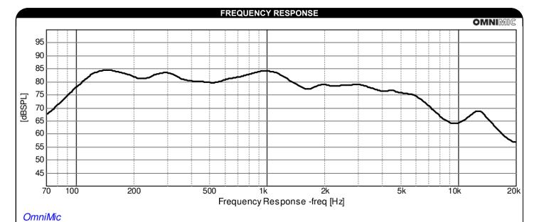
1/3<sup>rd</sup> octave smoothing - measurement taken with transducer adhered off-center on a 12" x 12" x ½" foam core board in an infinite baffle setup.
