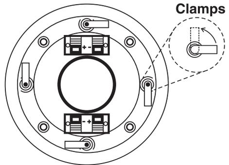
**CAUTION: Do Not Over-Tighten the Clamps. Too much torque may snap off the lug and the speaker will not seat securely. A snug fit is all that is necessary to assure proper performance.**
