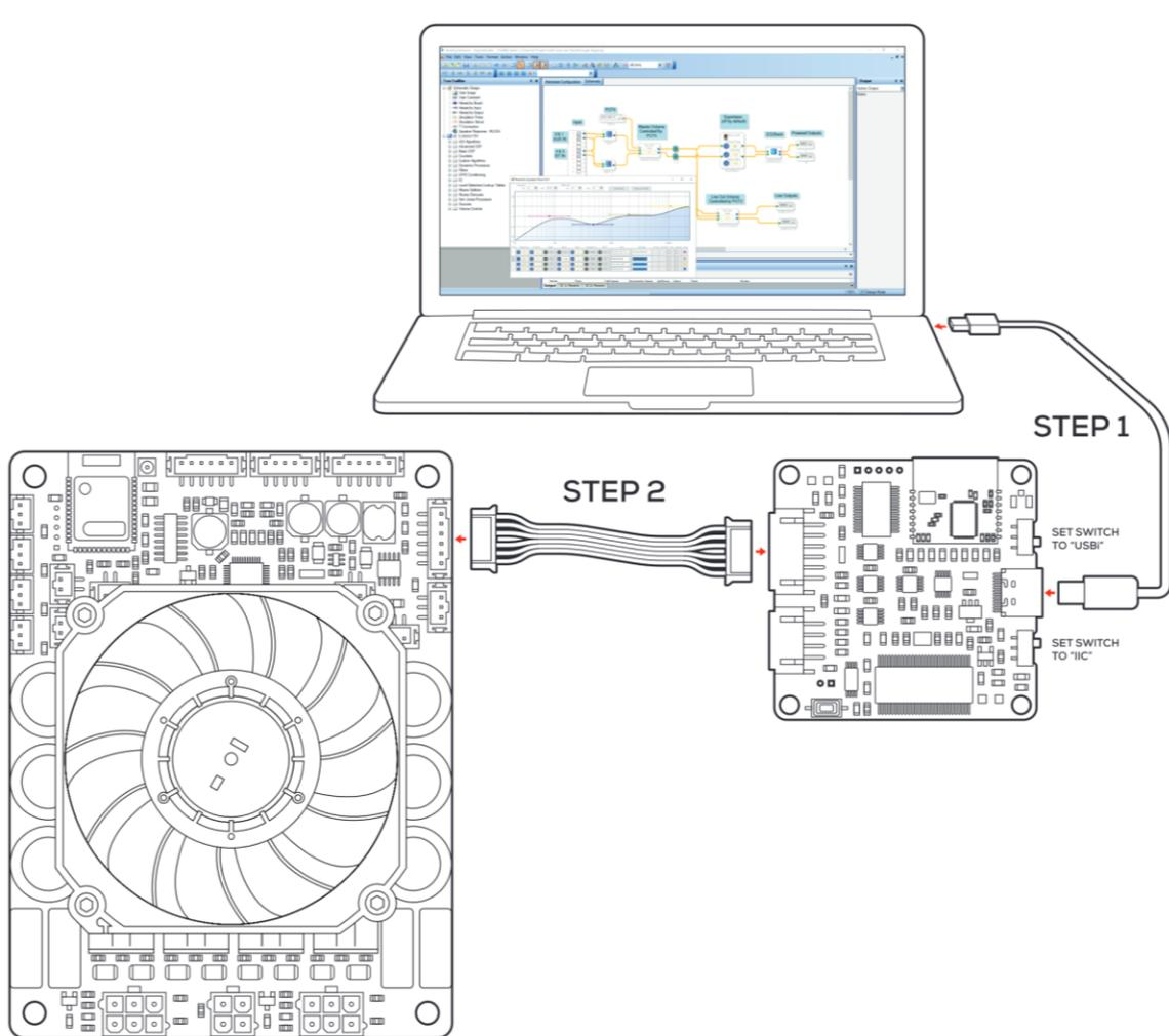
*The graphic above demonstrates using a KPX Programmer to connect the KABD-4100 to a laptop, however an ICP1 programmer will also work.*
