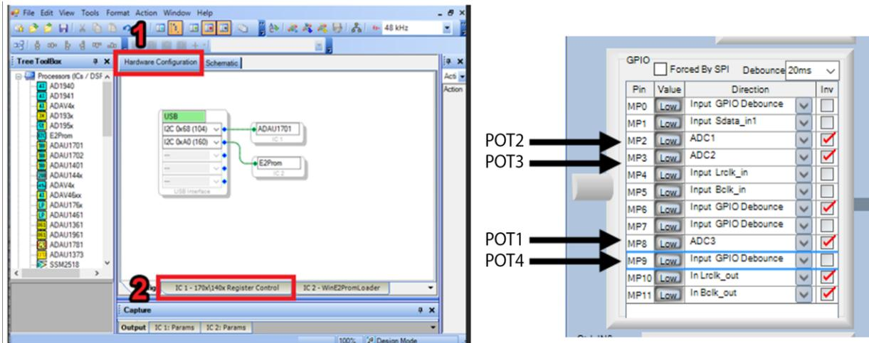
The screenshot shows the SigmaStudio interface. A red box labeled '1' highlights the Hardware Configuration menu. Another red box labeled '2' highlights the IC 1 - 170x\140x Register Control tab. To the right, a GPIO configuration table is shown with arrows pointing to specific rows:
