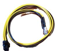
The SAB-1060 comes with a 4 pin molex mini-fit cable with a preinstalled female DC jack for easy connection to a power supply. If it is not needed, it can be cut off. This amplifier can be powered with a wide range of power supplies from 15V-30V, but for maximum stability, the 24V, 350 Watt MEANWELL LRS-350N2 or similar power supply is recommended. If less power is needed, a lower output power supply can be used as long as it is within 15-30V.
