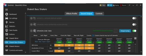
**Note:** If you are using front L and front R to power your game audio, do not assign any effects to channel 1 (front L) and channel 2 (front R). CH 3-8 are surround sound / sub outputs and should be used for bass shakers. If you are using the SAB-1060 as a dedicated sound card and have an external audio system, it does not matter which outputs you use for bass shakers.
