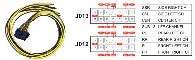
output. The chart above is from the perspective of each port from the top view of the SAB-1060.
