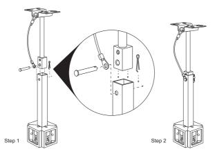
Part 2: Install the (4) QS204-4/QS204W-4 loudspeakers as shown.
